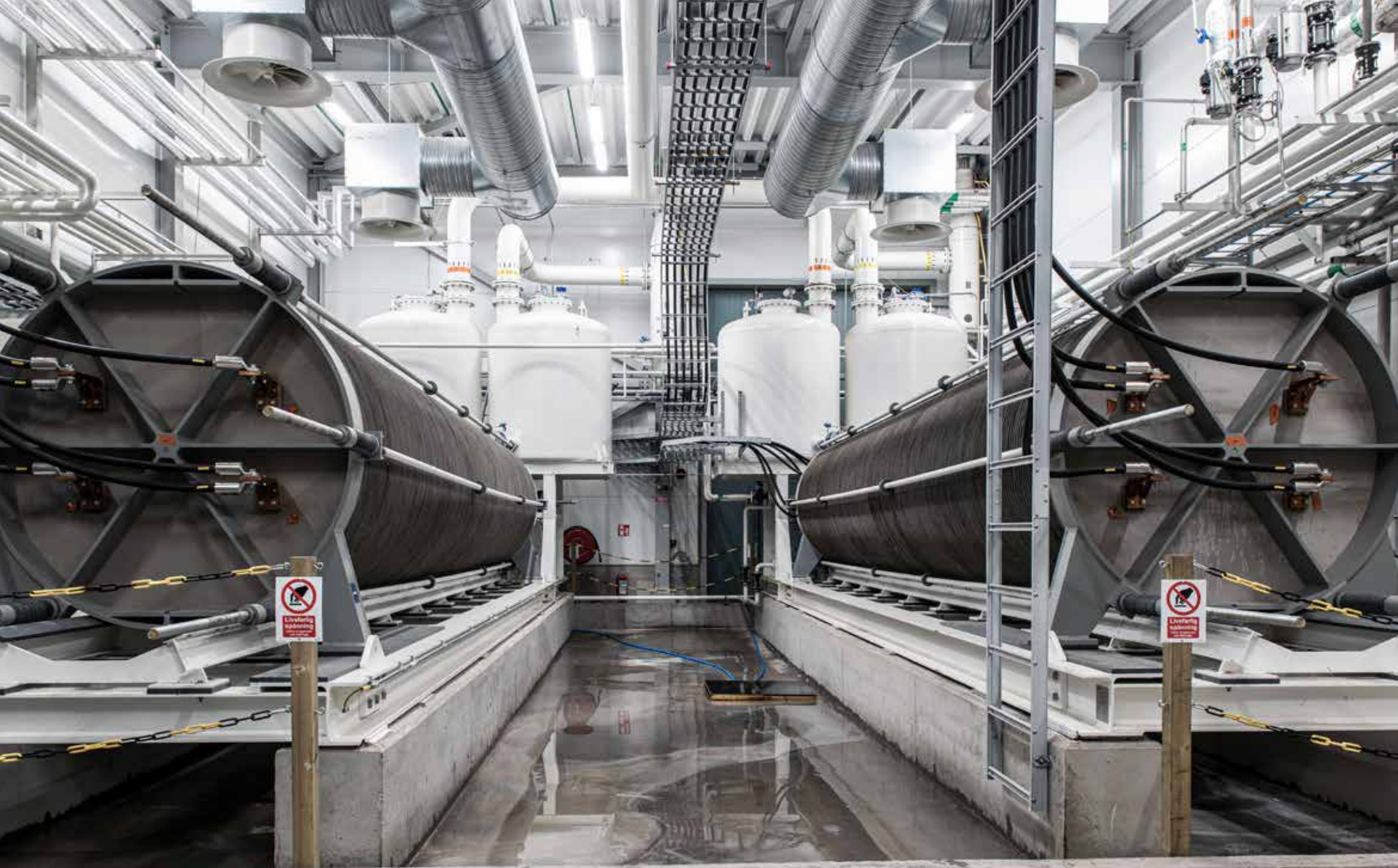
Alkaline electrolyzers using fossil-free energy produce all the hydrogen used in the direct reduction and hydrogen storage pilot plants.
